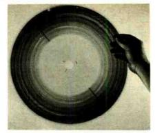
RECORDED DISC used with i/o Metrics system is 12 inches in diameter. The disc is capable of carrying in excess of one hour of video programming with a quadriphonic sound track,
