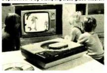
VIDEOPLAYER developed by Philips to play its VLP (Video Long Play) discs. Signal is fed to set's antenna terminals.
